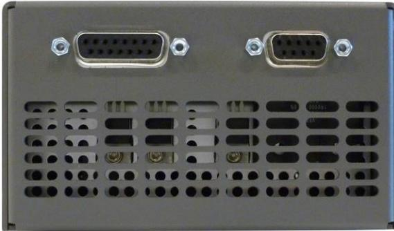
**ComboPak TEC (Left) and Laser (Right) Connectors**
